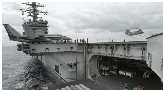
▲ ELEVATOR Four hydraulic lifts – one to port and three to starboard – move aircraft between the hangar and the flight deck. They also take stores or spare parts to and from the hangars.
